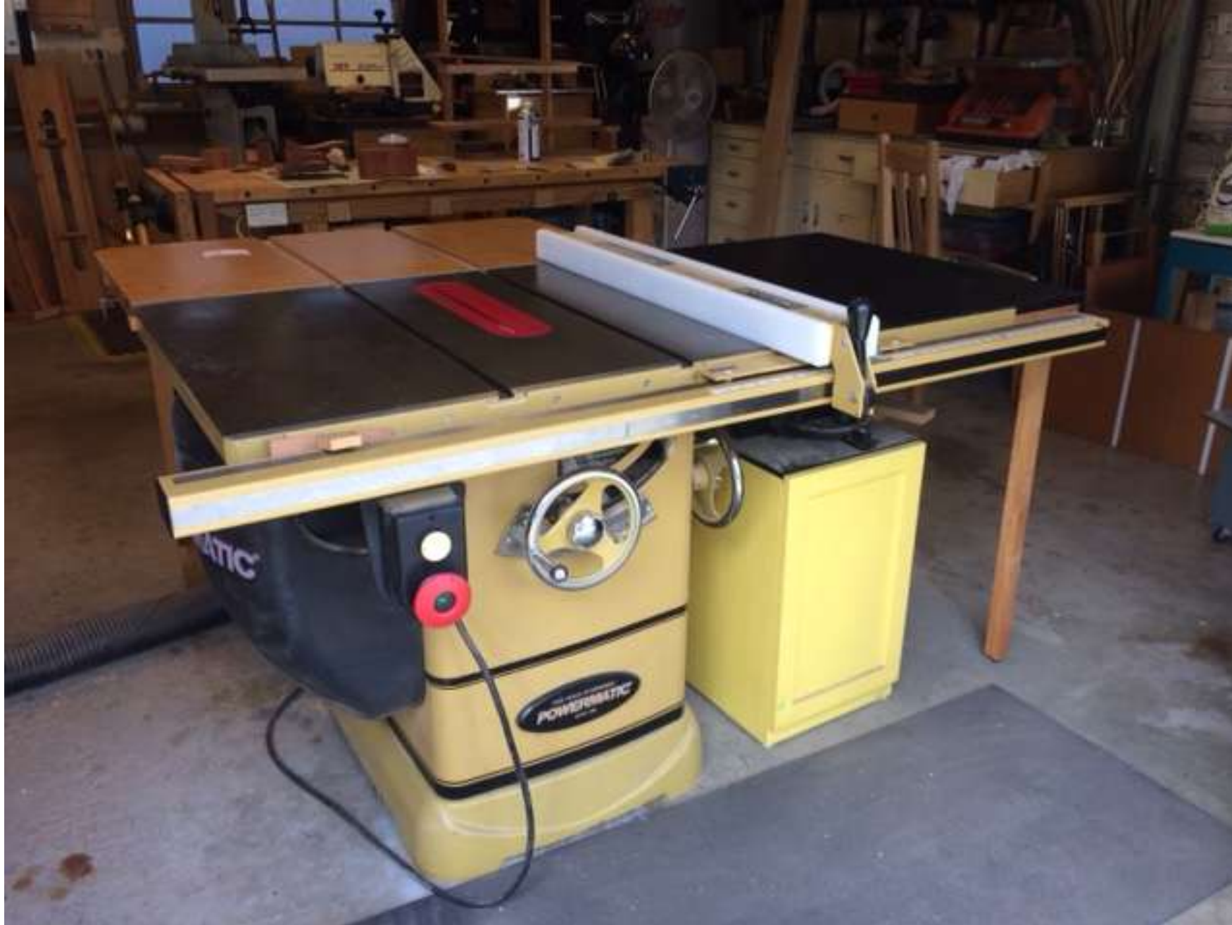
Powermatic 10" cabinet saw. It is equipped with an extension table and out feed table. The cabinet under the extension is for extra blades etc.
